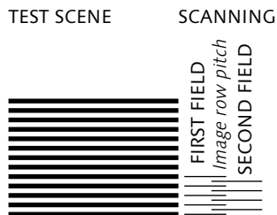
Figure 8.6 Twitter would result if this scene were scanned at the indicated line pitch by a camera without vertical filtering, then displayed using interlace on a short duty cycle display such as a CRT.
