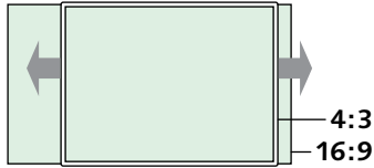
Figure 1.13 Pan-and-scan crops the width of widescreen material – here, 16:9 – for a 4:3 aspect ratio display.
