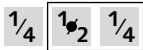
Figure 12.5 A cosited chroma filter for BT.601, 4:2:2 causes each filtered chroma sample to be positioned coincident – cosited – with an even-numbered luma sample.
